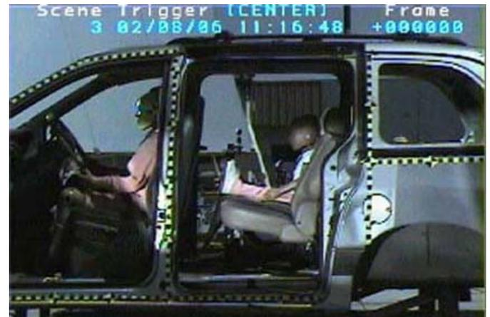
Fig 3. Corresponding Minivan Sled-Buck Configuration
