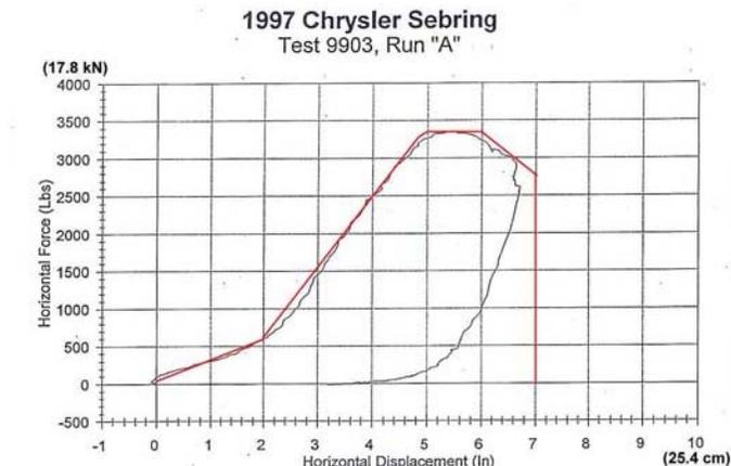
Fig 6. High Strength “belt-Integrated” Seat Data
