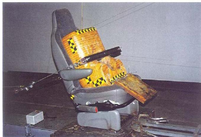
Fig 1. Quasi-static Body Block Strength Test Set-up
